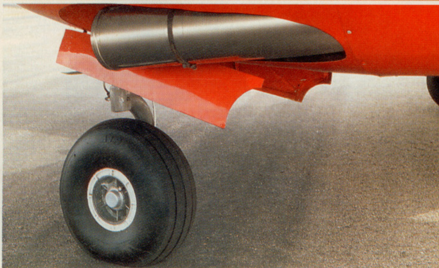
The engines exhaust through augmentor tubes (left), which eliminate the need for cowl flaps and give the Apache an authentic sound. N3369P's headset jacks are hidden in ashtrays and are connected to a new audio panel/intercom system (above).
